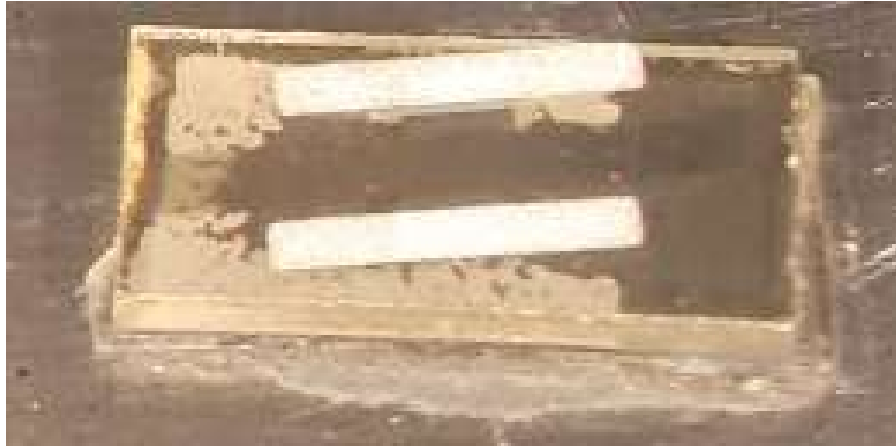
Figure 4.17 An image of one of the SAWR sensors mounted on static strain beam using Duralco 4525.
