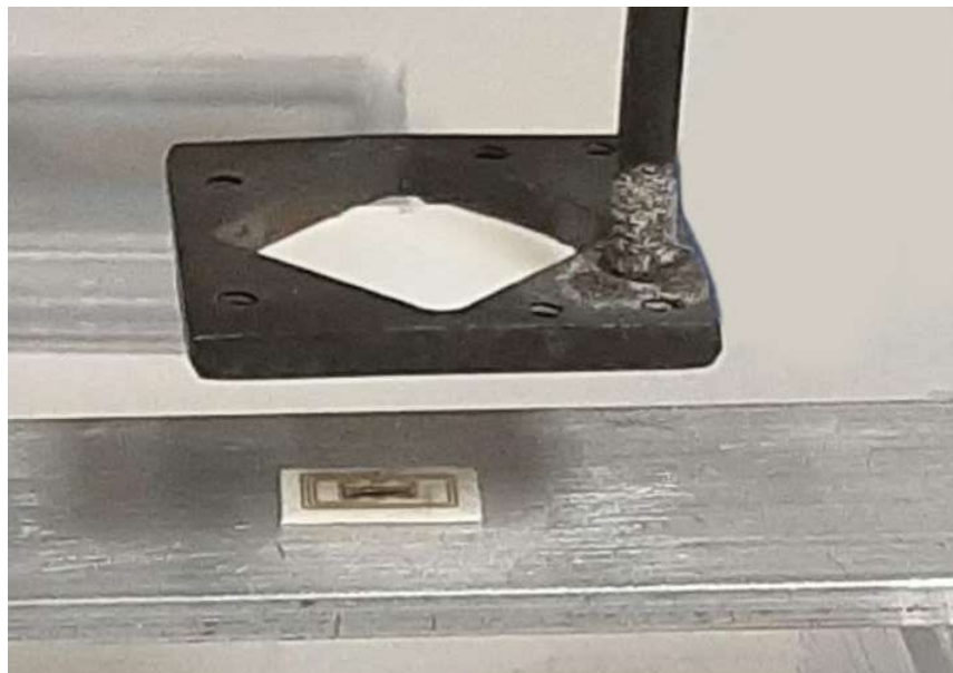
Figure 3.3 The interrogating antenna and sensor antenna used to interrogate the SAWR static and dynamic strain sensors [14].
