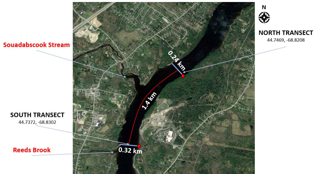
Figure 12: Penobscot River sampling site aerial with named tributaries. Locations of cross-channel ADCP origins (red circles) and transects (blue lines) are overlaid. Cross-channel distances and along-channel distance between the North and South transects are given in white.
