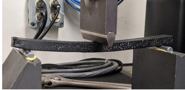
Figure 4.14: Control beam during three-point testing
