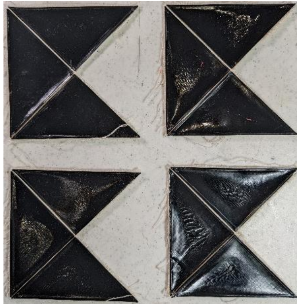
Figure 3.10: Additive manufactured models of the cube shelter concept, the short edge is 66 mm
