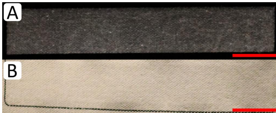
Figure 5.16: PMMA covered peel samples at 120°C
