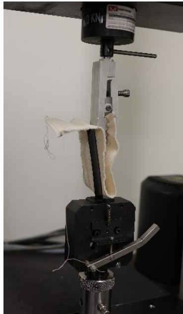
Figure 4.11: Peel sample setup (a) Peel sample infill orientation (b) Visual of created peel sample on cotton duck cloth (c) Peel test setup, black scale bar is 25 mm
