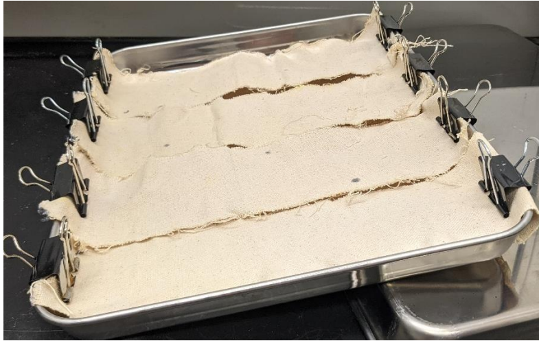
Figure 4.5: Drying setup for samples, samples would be clipped into place on a pan after having the coating applied to them as to prevent them from curling, pan would be put at an angle to prevent solution creating a thick coating on the bottom
