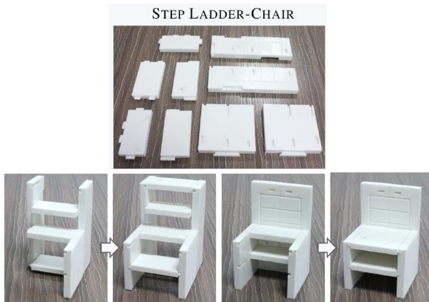
Figure 2.25: Additive manufactured step ladder chair made of nine parts that can be assembled as either a step ladder or a chair [24]
