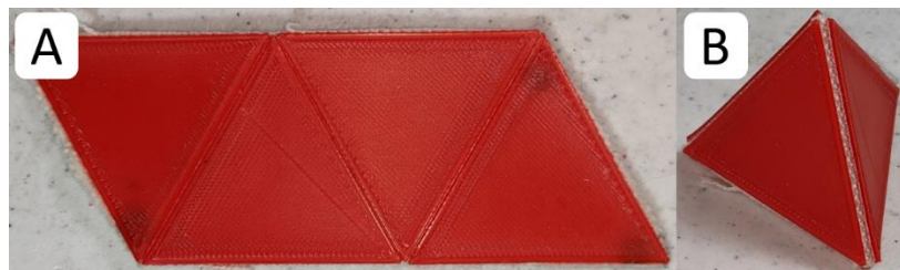
Figure 3.13: Created tetrakis hexahedron, (a) unfolded pattern with extra fabric still connected just after manufacturing, (b) faces cut away from the extra fabric, (c) erected object, short edge of triangles is 37 mm
