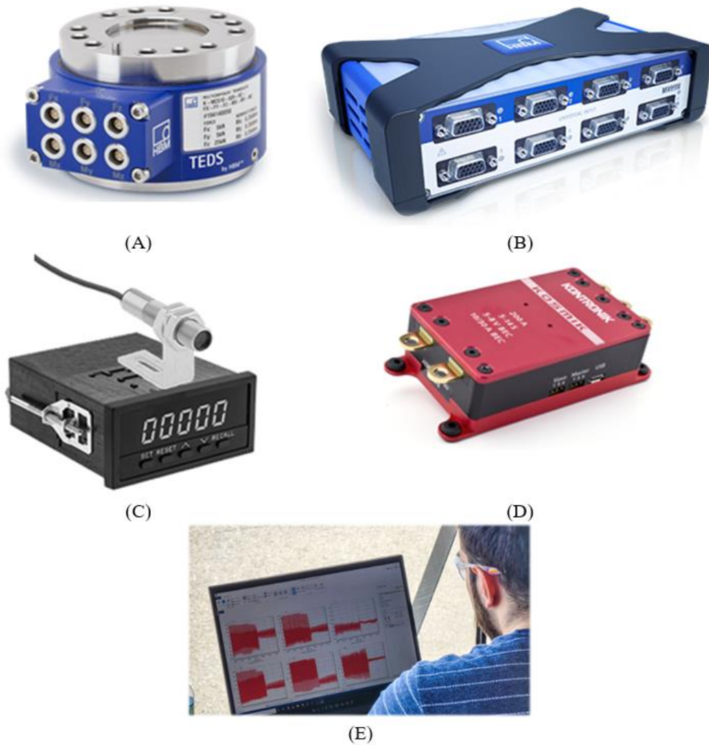
Figure 2.11 Load Cell (A). Quantum X (B). Tachometer setup (C). Speed Controller (D). Catman software environment (E).
