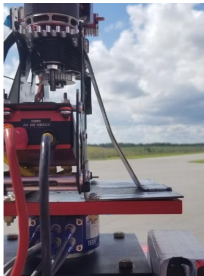
Figure 2.8 DEP pod design 1 supports buckle due to high vibrations
