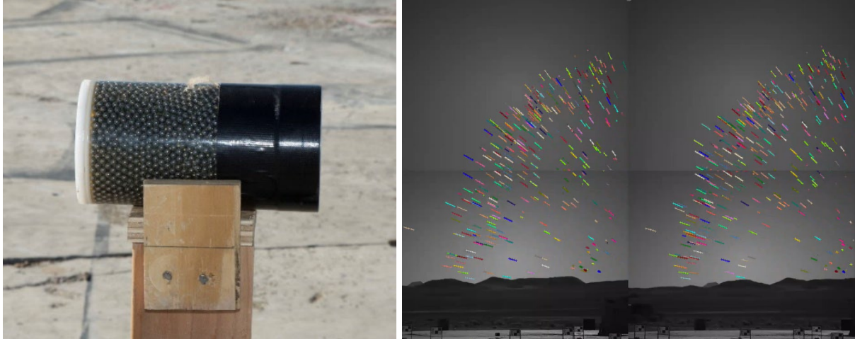
Figure 3.1 The experimental static arena test set-up for 5 mm ball bearing detonation (left) and fragment tracks from stereoscopic imaging (right).
