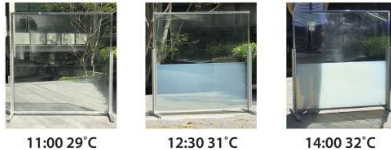
Figure 4-6 Smart thermoresponsive window treatment change opacity at surface temperature of 31°C (adapted from Zhou et al. 2020)
