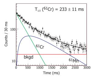
FIG. 3. (Color online) Decay curve for  ${}^{61}$ Cr, based on fragment- $\beta$  correlations. Data were fitted with a single exponential decay and exponential growth and decay of the short-lived daughter  ${}^{61}$ Mn ( $T_{1/2} = 670 \pm 40$  ms). A constant background was also considered in the fit.
