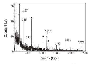
FIG. 4.  $\beta$ -delayed  $\gamma$  rays following the decay of <sup>61</sup>Cr. Known  $\gamma$  rays from the decay of the daughter <sup>61</sup>Mn and the granddaughter <sup>61</sup>Fe are indicated by the solid circles and squares, respectively. Transitions assigned to the decay of <sup>61</sup>Cr are marked by their energy in keV.
