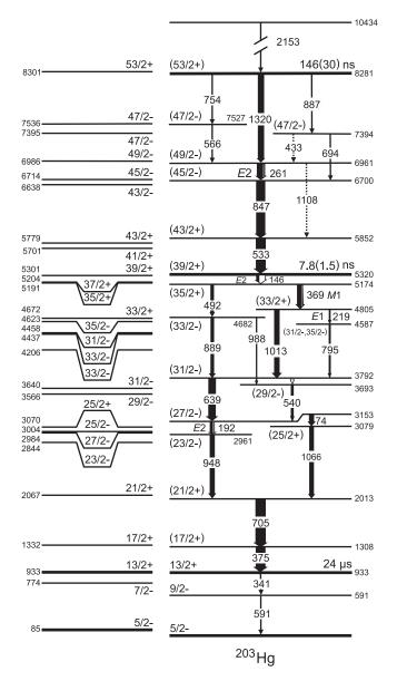
FIG. 3. Proposed decay scheme for the  $53/2^+$  isomer in  $^{203}$ Hg (right) compared with a shell-model calculation (left). The energies are relative to  $^{208}$ Pb, but the experimental ground state of  $^{203}$ Hg is set to zero. Transition intensities are indicated by the width of the arrows.
