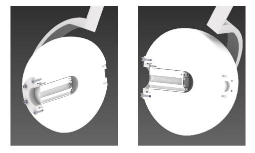
**Figure 1.** Schematic drawing of a low-Z chamber made from a Bonner sphere. This sphere was designed to maximize the coverage with a low-Z material while minimizing the attenuation of  $\gamma$  rays. The beam enters for the left side, and impinges on the target, located in the middle. The target is removable and is easily slid in and out. The sources used for efficiency calibrations were placed in the target position before and after the run was completed.
