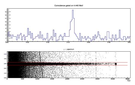
**Figure 2.** Coincidence spectrum accumulated from the  $TiD_2$  target displayed together with the projection from the gated 4.44-MeV peak on top; the energies are binned in 0.666 keV/channel. The 4.44 MeV (ch. 2961) gated spectrum clearly shows a peak at 3.21 MeV (ch. 2142).
