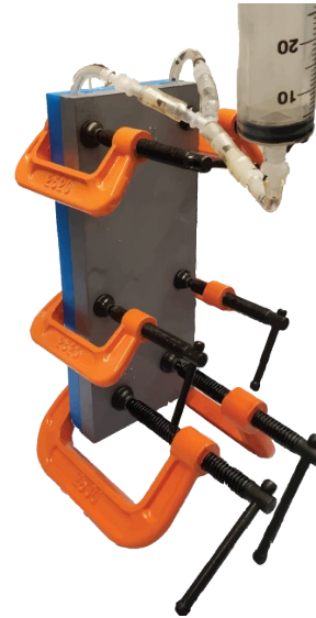
Figure 11: Casting injection configuration. A 50-milliliter syringe was used to inject casting material into the clamped mold.
