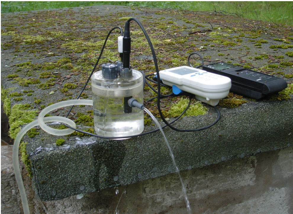
Figure 5 Making well-head measurements using a flow through cell.
