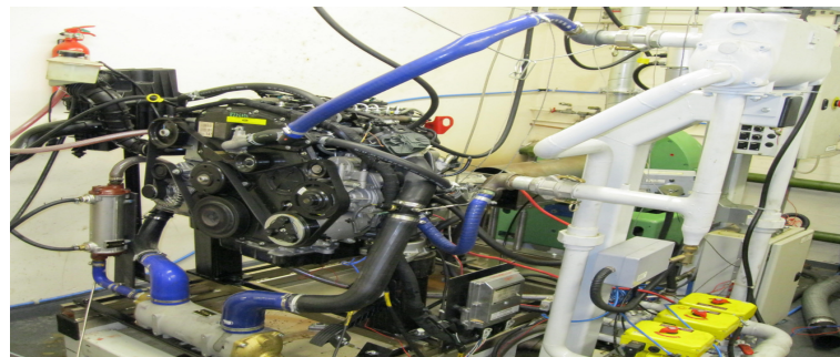
Figure 4. Typical view of Ford Puma Engine as used in testing
