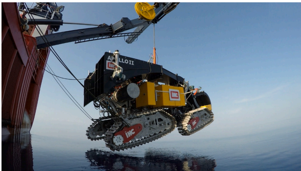
Fig. 2. Deployment of the Apollo II pre-prototype nodule collector vehicle from the aft of RV Sarmiento de Gamboa during the 2018 field test in Málaga Bight. Photo courtesy: Alberto Serrano. Note the Nortek Aquadopp current profiler mounted upward-facing on starboard side of the diffuser. Acoustic backscatter data presented in Fig. 11E were acquired with the current profiler mounted backward-facing.
