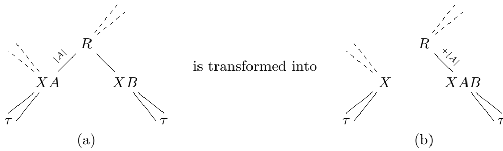
Figure 3: (a) Transformation preconditions: all trees \tau at the right node have copies at the left node and the weight of the left edge equals |A| ; (b) result of the transformation.
