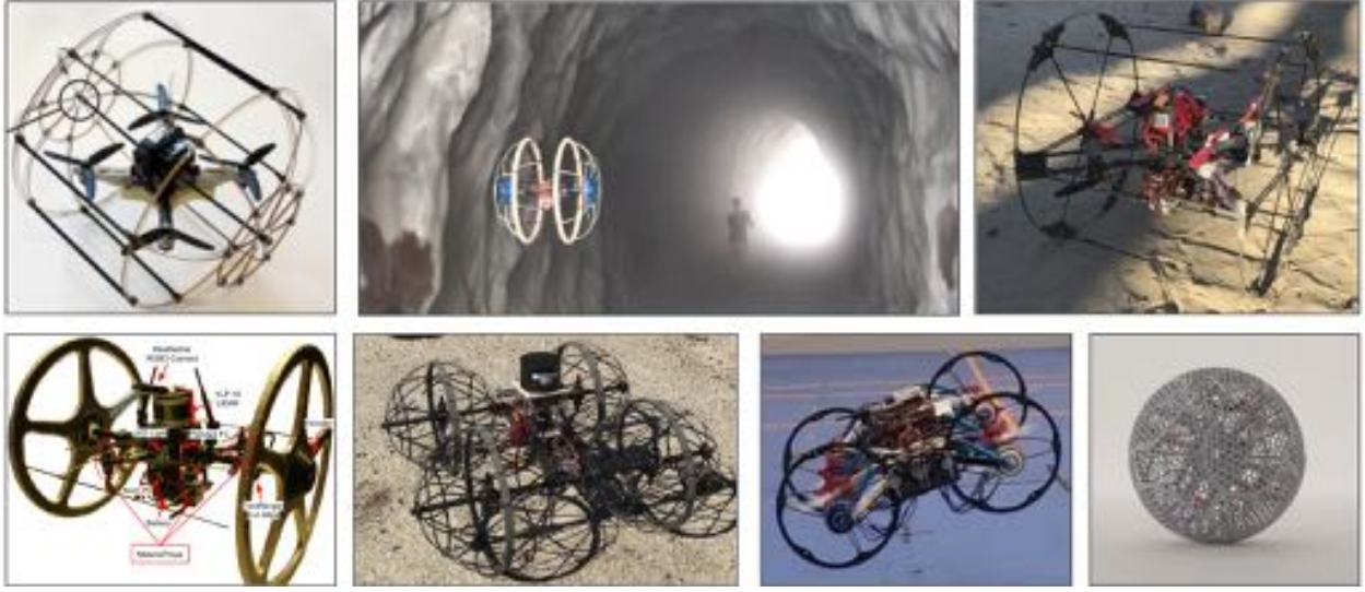
Figure 50: Hybrid platform hardware evolution (top row: left to right) pre-challenge Hytaq design [Kalantari and Spenko, 2014], Modular hybrid vehicle [Agha-mohammadi et al., 2020], (bottom row: left to right) Autonomous Rollocopter [Fan et al., 2019, Lew et al., 2019], DrivoCopter [Kalantari et al., 2020], BAXTER [Choi et al., 2020], Spherical Rollocopter [Sabet et al., 2020, Sabet et al., 2019].
