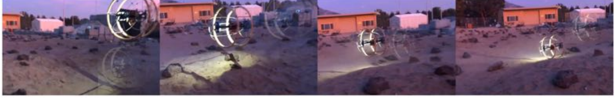
Figure 49: Hybrid platform flying over an obstacle at the JPL Mars Yard [CoSTAR Team, 2018a].
