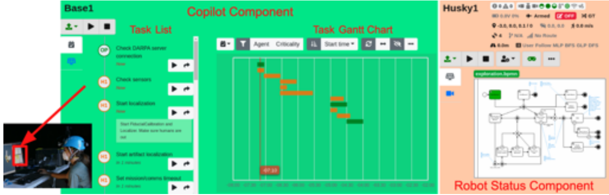
Figure 39: Base station single screen setup and human supervisor interacting with the user interface (left). Autonomy assistant Copilot MIKE’s interface component with task list and Gantt chart mission overview (middle). Robot status component displaying the robot’s state in the exploration mission (compare Figure 38), real-time information regarding sensor hardware, current pose and other housekeeping data that represents current beliefs (right).
