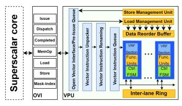
Fig. 1. VPU is connected to the Scalar Core through OVI.
