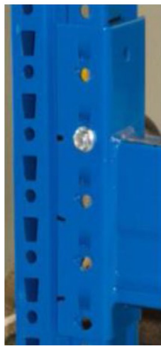
(c) Beam-to-upright hooked connection with a bolt
