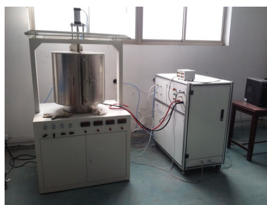
Fig. 6 – 3 kW Solid Oxide Fuel Cell stack testing system
