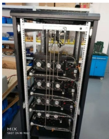
Fig. 5 – Power system with 4 kW fuel cells to study the possibilities of use on ship
