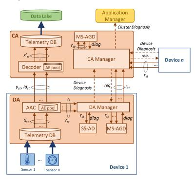
**Figure 2.** Detailed architecture and key components.
