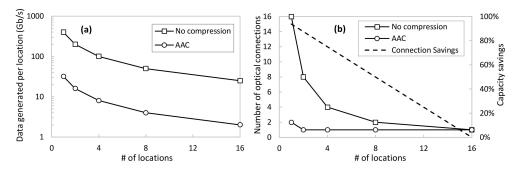
Figure 10. Network study analysis: data generated (a) and number of optical connections (b).
