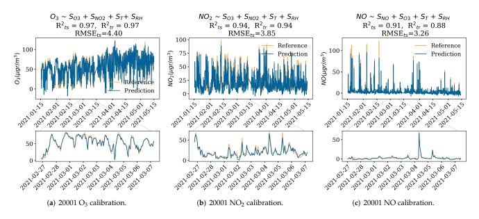
**Figure 4.** Calibration results for the  $O_3$ ,  $NO_2$  and NO sensor of Captor nodes 20001 and 20002.  $R_{ts}^2$  and  $R_{tr}^2$  denote the training and testing coefficient of determination, while  $RMSE_{ts}$  denotes the root-mean-squared error for the testing using MLR. Bottom plots are a zoom of the plots above for a specific time interval.
