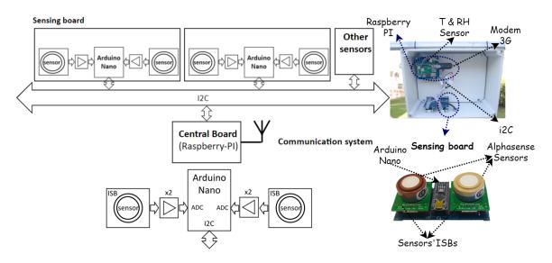
**Figure 1.** Air pollution data capture prototype Captor node on (**top**), and the Captor's sensing board on (**bottom**). The prototype node has a Raspberry-based central processing unit connected to the sensing boards via an I2C bus. Each sensing board has an Arduino Nano microcontroller unit in charge of collecting the measurements from the electrochemical sensors and sending them to the Raspberry unit. The collected samples are then transmitted to the cloud via a 3G modem.
