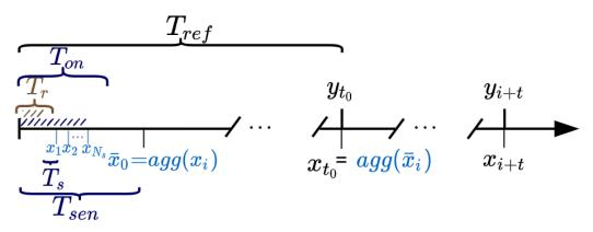
**Figure 3.** Sensor sampling scheme used throughout the article.  $x_i$  are the sensor measurements while  $y_i$  are the reference data measurements. Every  $T_{sen}$ , the sensor is sampled by waiting for the sensor response time  $T_r$  and collecting the  $N_s$  samples to be aggregated. These  $T_{sen}$  samples can be further aggregated into  $T_{ref}$  to synchronize them with the reference values.
