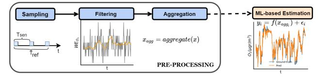
**Figure 2.** Sensor data gathering pipeline: from sensor sampling to machine learning estimation. First, sensors are sampled every  $T_{sen}$ , then the samples collected during this period are filtered to eliminate possible outliers and aggregated to be sent to the cloud. There, the air pollution concentrations are estimated using the calibration models.
