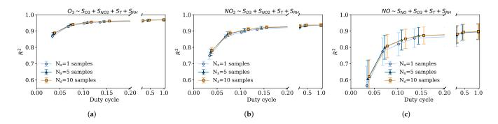
**Figure 7.** Average CV R<sup>2</sup> and 95% confidence intervals for different duty cycles with a sensor response time equal to 2 min ( $T_r = 2 \text{ min}$ ) using MLR. (**a**) Captor 20001 O<sub>3</sub> CV R<sup>2</sup> for different duty cycles. (**b**) Captor 20001 NO<sub>2</sub> CV R<sup>2</sup> for different duty cycles. (**c**) Captor 20001 NO CV R<sup>2</sup> for different duty cycles.
