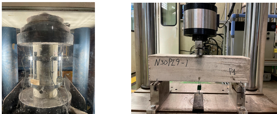
Figure 4. Experimental testing: stress–strain relationship (left); residual tensile strength (right).
