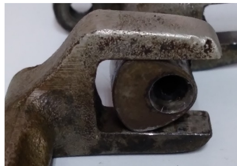
Figure 2. Photograph of the constant-breadth cam mechanism with a flat-faced double-oscillating follower, used in a traditional sewing machine.
