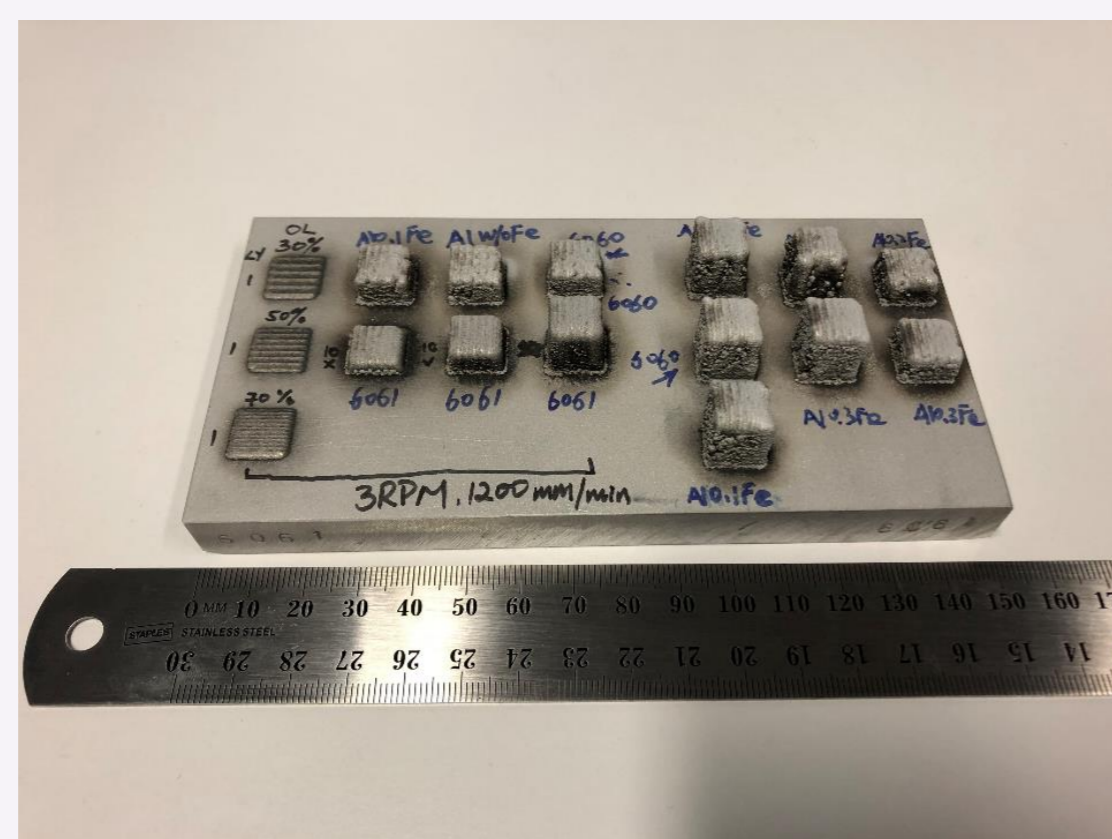
Part produced via Direct Energy Deposition process. 1
