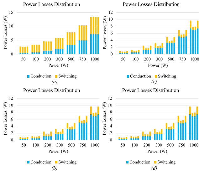
FIGURE 5. Power losses distribution of (a) PSPWM, (b) IPD, (c) POD, and (d) APOD. The power losses are grouped in sets of 4 bars each, a bar per half-bridge module: (from left to right) module 1 to module 4.
