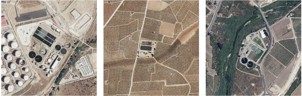
Figure 1. WWTPs present broad differences in their visual appearance. However, in orthophotography, they usually stand out by their circular and rectangular-shaped infrastructures. These and Figure A1 images correspond to very high-resolution crops from the Spanish National Geography Institute (IGN).
