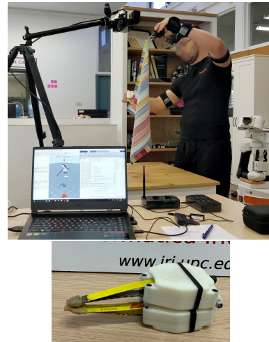
Figure 4: Experimental setup. (Top) The subject wears a motion tracking suit, a GoPro camera mounted on the head and we also take a Kinect screenshot of the final result, although the latter is not used in this paper. (Bottom) Wearable point-point gripper used in the experiments.
