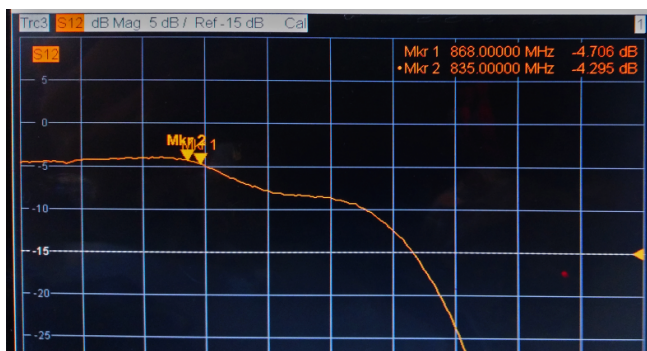
Figure 3.33: S_{12} parameter with VNA
