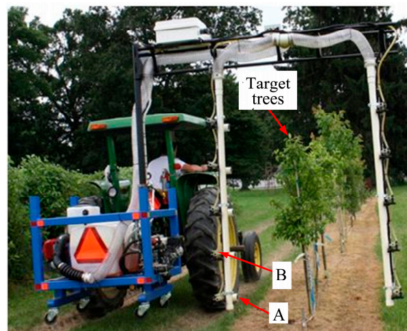
Figure 13. The real-time variable-rate sprayer and its components (A—ultrasonic sensor, B—spray nozzle with PWM solenoid valve) [111].
