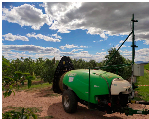
Figure 15. Prototype of the variable-rate sprayer developed in the European OPTIMA project.
