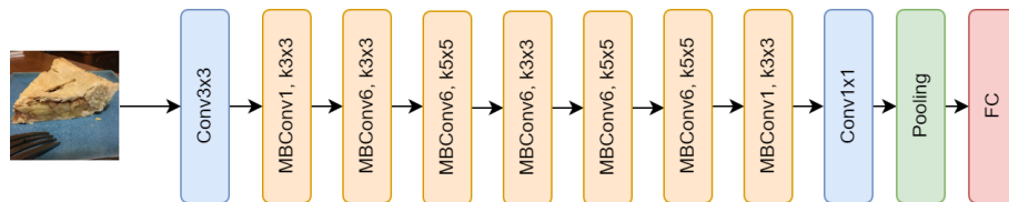
Figure 3.4: Diagram showing the structure of the generic EfficientNet [55] architecture.
