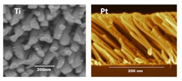
Top view (left) and cross-section (right) SEM images of Ti and Pt NCFs, respectively.
