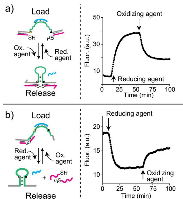
Figure 5. Reversible redox-controlled ligand release and loading. (a) Reversible release and loading of the ligand ( 5 \times 10^{-8} M) from the nanodevice ( 3 \times 10^{-8} M) upon reduction and successive oxidation of the redox disulfide inhibitor ( 3 \times 10^{-7} M). (b) Reversible
