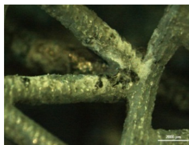
(e) Porosity of the foam, 100× optical microscopy.
