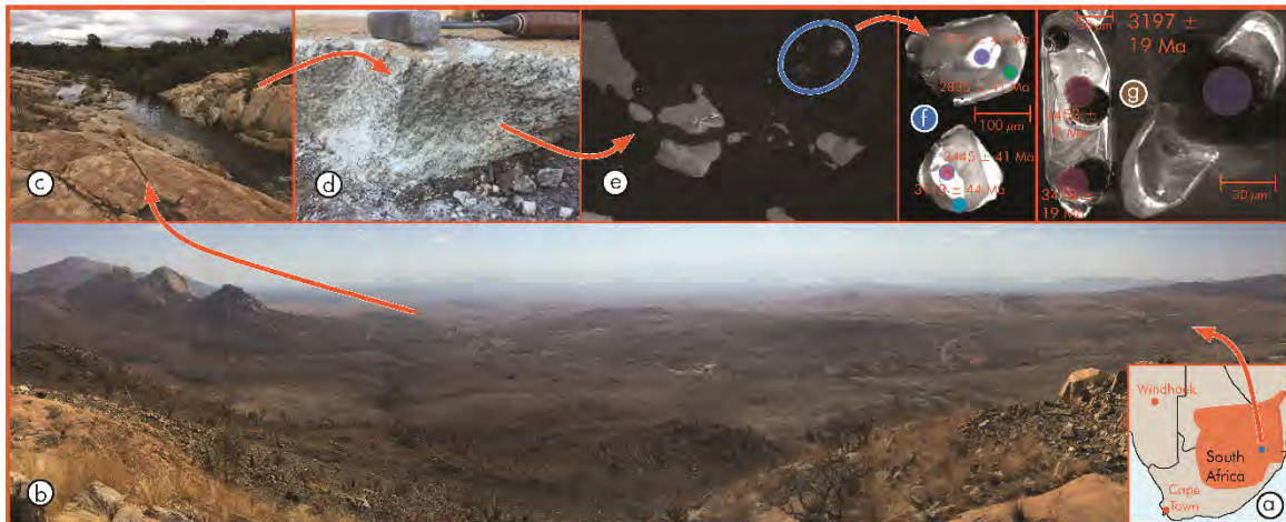
Fig. 1 (above). From macro to micro: (a) location of the Kaapvaal Craton and the study area -> (b) study area, the Stolzburg Block -> (c) outcrop -> (d) sample -> (e) thin section -> (f) apatite and zircon crystals. Fig. 2 (right). The principle behind thermochronology of apatite [ \text{Ca}_5(\text{PO}_4)_3(\text{OH},\text{F},\text{Cl}) ] and zircon [ \text{ZrSiO}_4 ], the closure temperature ( T_c ). Some Ca in apatite and some Zr in zircon can be replaced by U, which decays into lead at a half life of ca. 4.47 billion years for ^{238}\text{U} and ca. 704 million years (Ma) for ^{235}\text{U} . Above T_c , the crystals equilibrate with their surroundings and Pb is lost. When a crystal cools below T_c , the isotopic clock starts ticking, and the age obtained by isotope analysis reflects that time. Metamorphic crystals can grow beneath T_c , but can be identified with the electron microscope (Fig. 1f+g).
