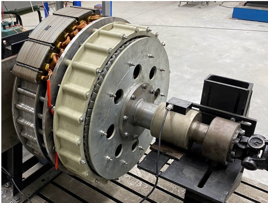
Figure 6.6: Prototype 15 kW SS-PMG on the testbench connected to a 5000 Nm torque sensor.
