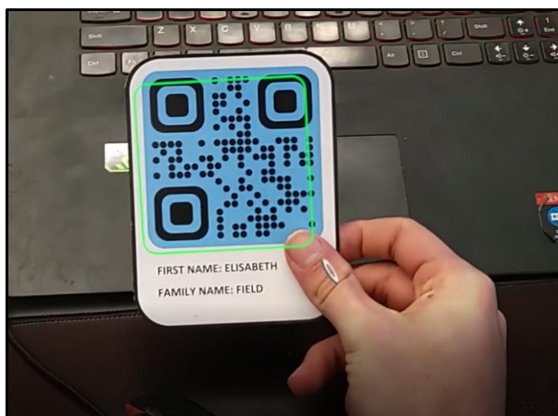
Figure 50: Screenshot of the QR scanning using the Microsoft HoloLens 2 augmented reality device.
