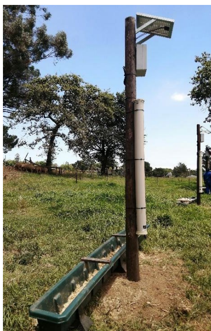
Figure 3.3 An indication of the LoRa methane detection units installed in the camp, on the Welgevallen Experimental Farm, on 4m poles for the duration of the study.
