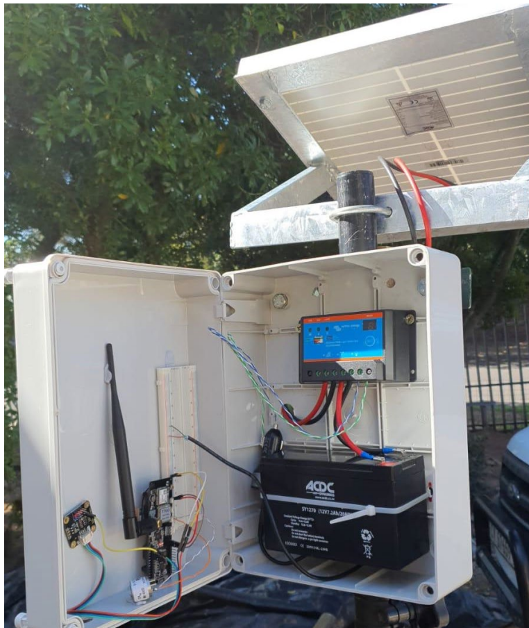
Figure 3.1 An indication of the different components of the LoRa methane measurement units that was located in the camp on the Welgevallen Experimental Farm, throughout the study period.
