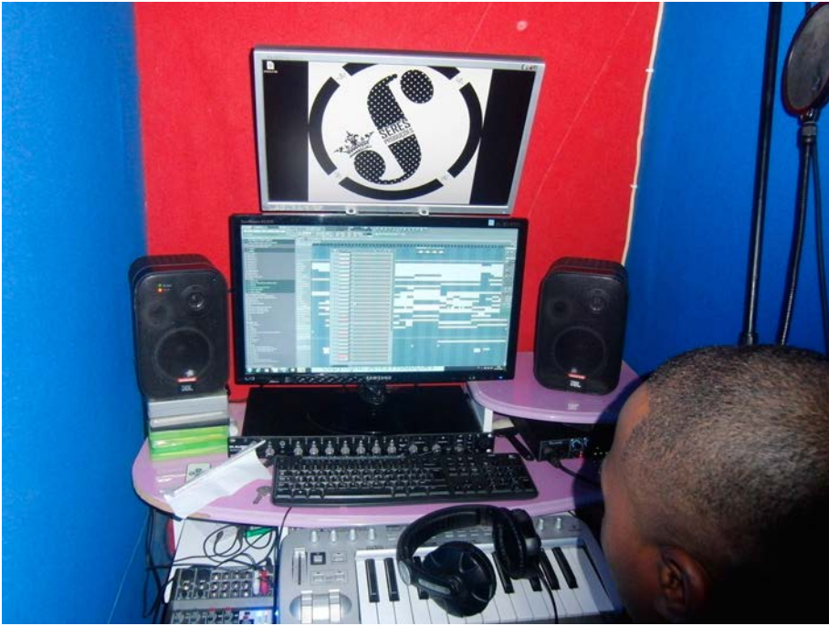
Figure 1 Studio of Seres Produções run by DJ Satelite, Luanda, 2012—Studio of Seres Produções run by DJ Satelite in a storeroom in a residential building. On the bottom screen a work-in-progress afrohouse track in FL Studio software. Top screen shows the produtora’s logo. The set-up comprises desktop PC, a two octave keyboard as MIDI controller, two monitor speakers, external audio interface, two screens, an effect rack (under bottom screen), headphones, five channel mixing board (left of keyboard), and microphone with pop filter (far right). Marçal, Luanda, 2012. Photo by the author.
