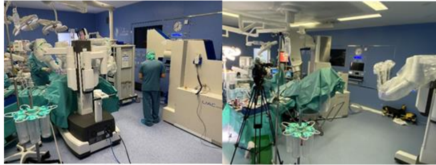
Figure 1. A modern operating room with a miniaturized-mobile electron linear accelerator and a robotic Da Vinci system used together to treat a prostate cancer patient with IOeRT (post-resection of oligonodal relapse) Liac HWL, Sordina IORT Technologies.
