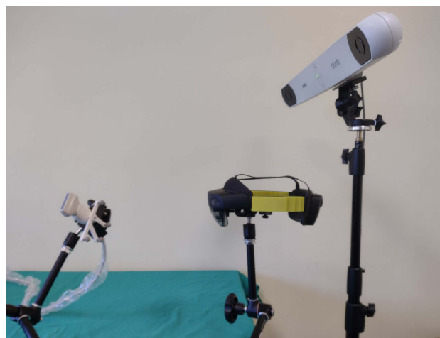
Fig. 4 Setup for the static tracking accuracy evaluation. HoloLens 2 and the OTS are fixed, while the US probe with its marker is moved to 20 different poses for measurement acquisition
