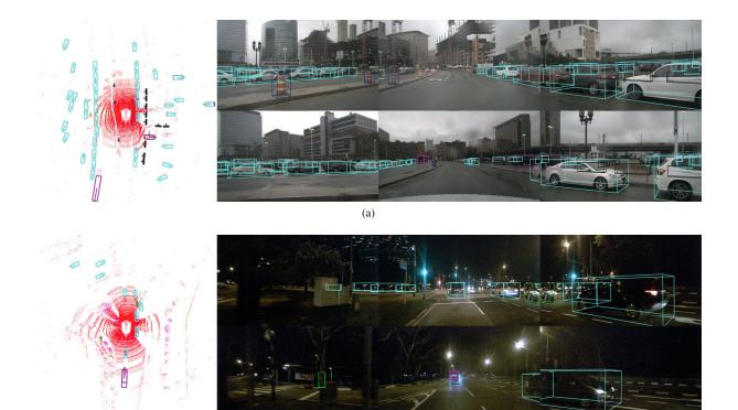
FIGURE 12. Results of BirdNet+ with rainy and night conditions on the nuScenes test set. Detections in the BEV are shown on the left. The RGB images correspond to the front-left, front, front-right, rear-left, behind, and rear-right cameras, respectively.
