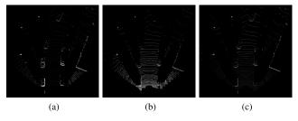
**FIGURE 2.** Baseline BEV feature encoding: (a) Maximum height. (b) Mean intensity. (c) Normalized density. Contrast corrected for visualization.
