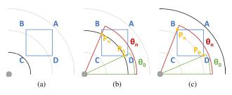
**FIGURE 3.** Horizontal cross-section of possible LiDAR-cell intersection scenarios: (a) No intersection. (b) LiDAR ring intersects with the upper/lower plane of the 3D pillar. (c) The cell is fully intersected by the laser plane.
