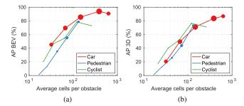
FIGURE 8. Detection performance vs. average number of cells spanned by an object on the KITTI validation subset (Moderate difficulty): (a) AP BEV (%). (b) AP 3D (%). The radius of each marker is proportional to the number of objects.
