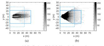
**FIGURE 7.** Spatial distribution of labeled objects in the KITTI dataset (Hard difficulty), represented in grid maps with  $2 \times 2$  m cells: (a) Total number of objects. (b) Mean number of 3D points per object. In both cases, rectangles in blue represent the area spanned by the former  $35 \times 70$  m BEV representation (dashed line), and the proposed BEV  $50 \times 45$  m representation (solid line).
