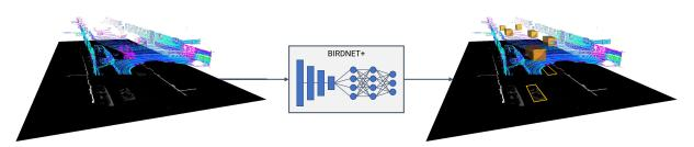
**FIGURE 1.** Input/output data involved in the BirdNet+ detection framework. The raw LiDAR point cloud is projected onto a BEV image where each pixel contains information of a 3D pillar. This BEV is fed to our CNN-based model that generates a set of fully parameterized 3D bounding boxes.
