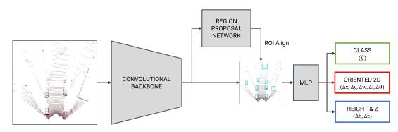
FIGURE 4. Overview of the proposed 3D object detector.
