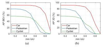
FIGURE 9. Detection performance vs. IoU threshold on the KITTI validation subset (Moderate difficulty): (a) AP BEV (%). (b) AP 3D (%).
