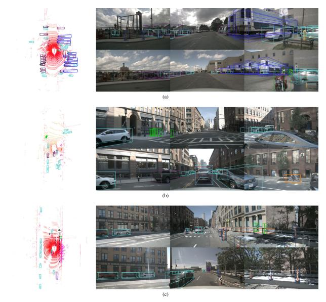
FIGURE 11. Results on the nuScenes test set. Detections in the BEV are shown on the left. The RGB images correspond to the front-left, front, front-right, rear-left, behind, and rear-right cameras, respectively.
