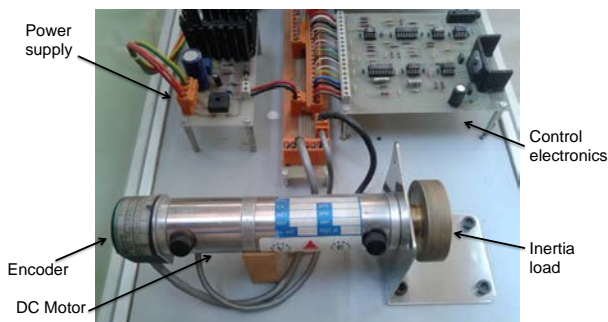
Figure 2: Real DC motor used in the experiments
