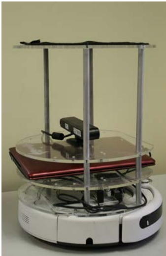
Figure 9. Turtlebot robot used as mobile platform for the inspection system
