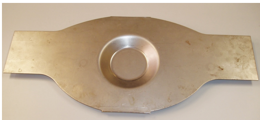
FIGURE 5: Deformed blank obtained by pattern test.
