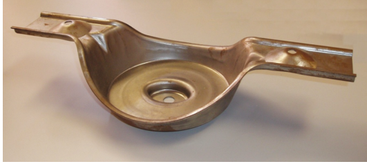
FIGURE 1: Part manufactured by five stamping stages.
