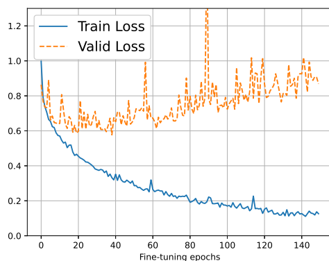
Figure 2.6: Fine-tuning a six layer MLP for FMNIST with dropout in all layers.
