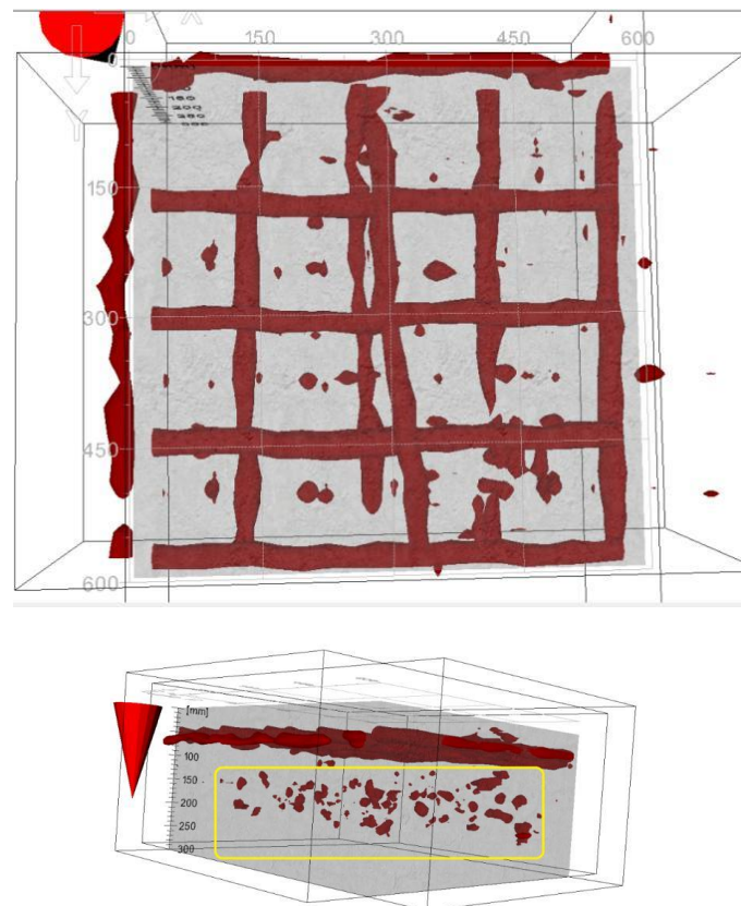
Figure 44- 3D view of 1st scan of Side -A showing the rebar details and other metallic object or voids
