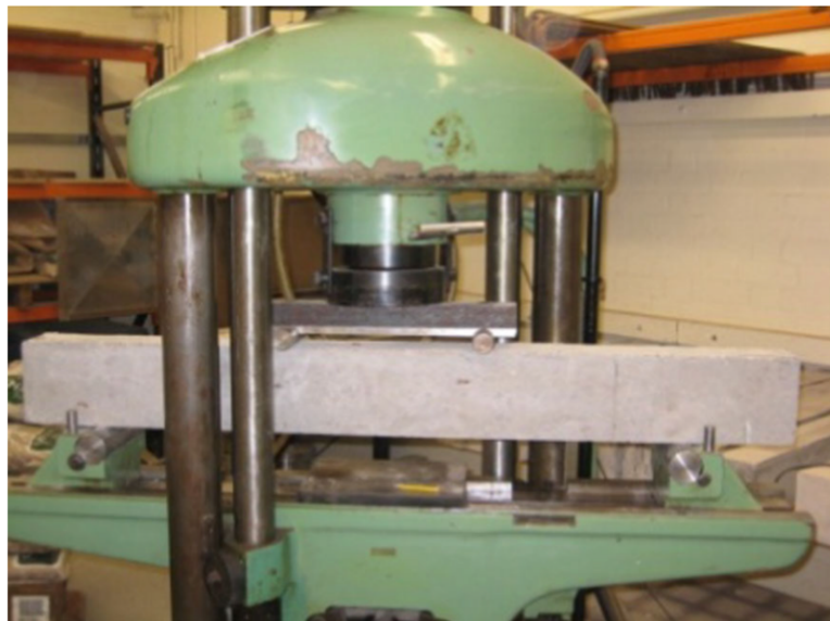
Figure 7: Bend test setup for rubber-filled concrete [15]
