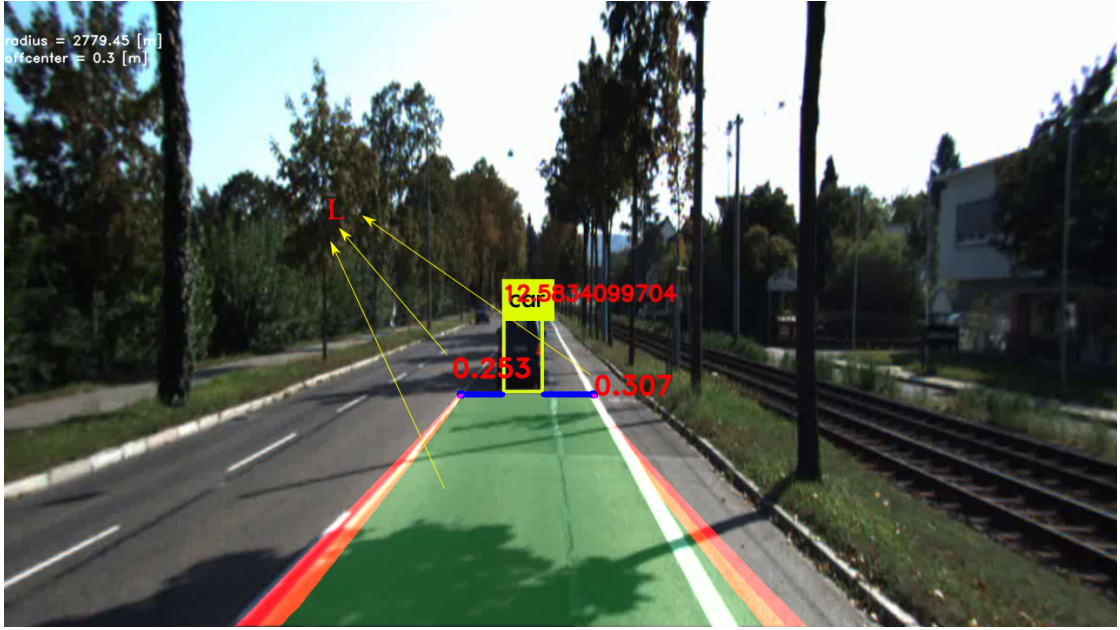
Figure 2.27: Estimated lane T_{\text{car}} is currently in, is shown by red boundaries. Number at top of the bounding box is distance of the detected car from ego vehicle in metres. Two fractional numbers at bottom of the bounding box are the distance of T_{\text{car}} from the nearest lane markings respectively in metres. Dividing these two values will give the relative lane position.
