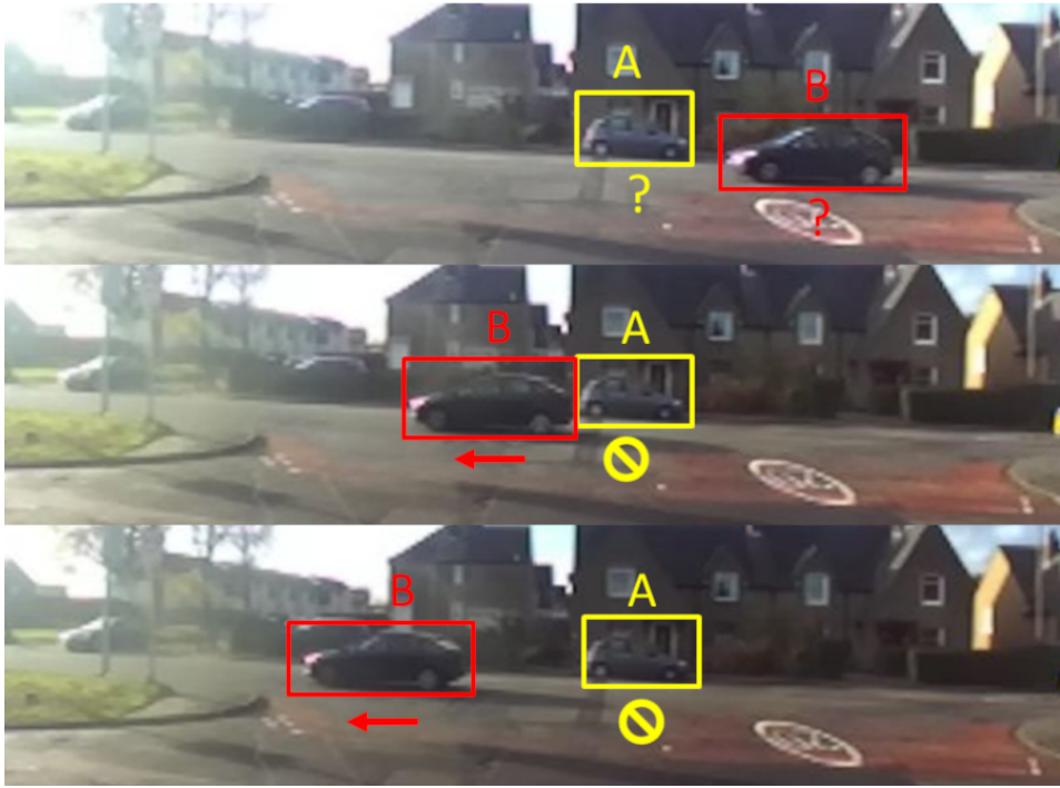
Figure 2.6: A typical example of a survey performed to understand the importance of video sequence instead of a single image frame to judge a vehicle’s motion and movement direction [91].
