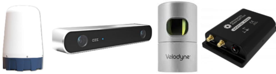
Figure A.3: All four sensors used in our test vehicle. Starting from left CTS350-X Navtech Radar, ZED Stereo Camera, Velodyne HDL-32E LiDAR and Advance Navigation Spatial Dual Kit.
