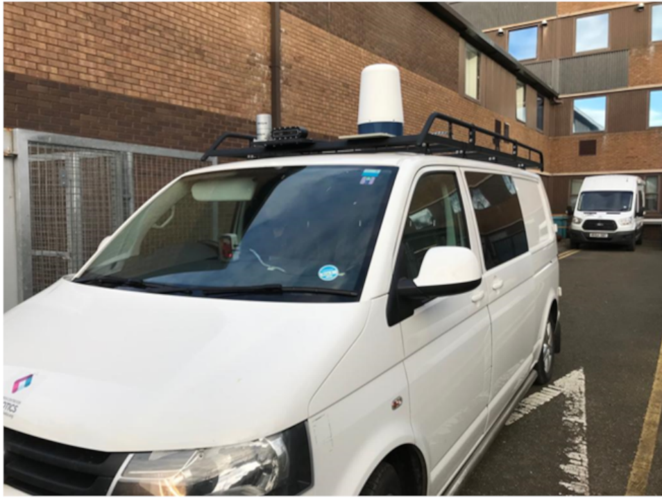
Figure 1.2: Sensor equipped test vehicle used to collect data. A detailed schematic diagram of the test vehicle specifying where each of the sensors are installed, their specifications and end-to-end data collection pipeline is explained in Chapter 3 or Appendix.
