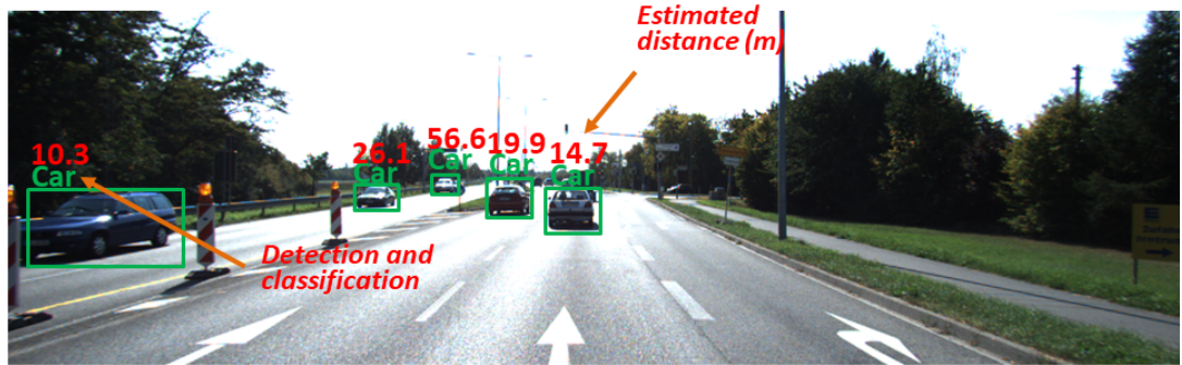
(b) Detection and classification of traffic participants in the scene. The bounding boxes are the detected target cars in the scene and the numbers in red are distances of the target cars from the ego vehicle in metres.
