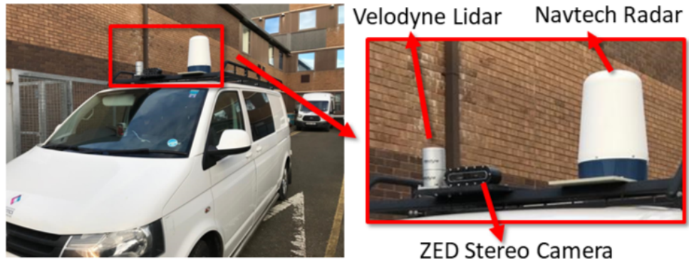
Figure 2.22: Test vehicle equipped with Velodyne LiDAR, Navtech Radar, ZED Stereo Camera and Advance Navigation GPS/IMU kit, used to collect data from different junction.
