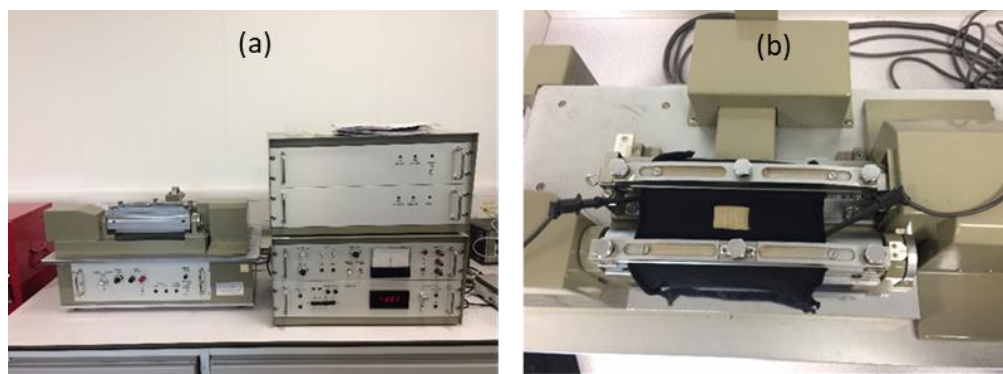
Figure 6.5 - Shear measurement, (a) KES shear instrument (b) shear experimental set up.
