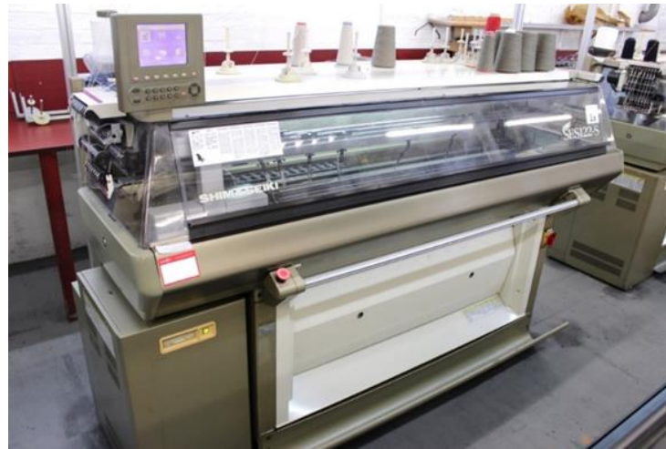
Figure 3.5 - Computerised flat-bed knitting machine, Shima Seiki SES 122-S 12 gauge.
