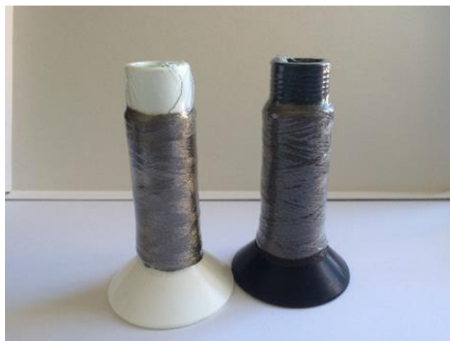
Figure 3.1 - Conductive threads: Silver plated nylon 117/1/ two-ply (left) and Silver plated nylon 235/34 four-ply (right).
