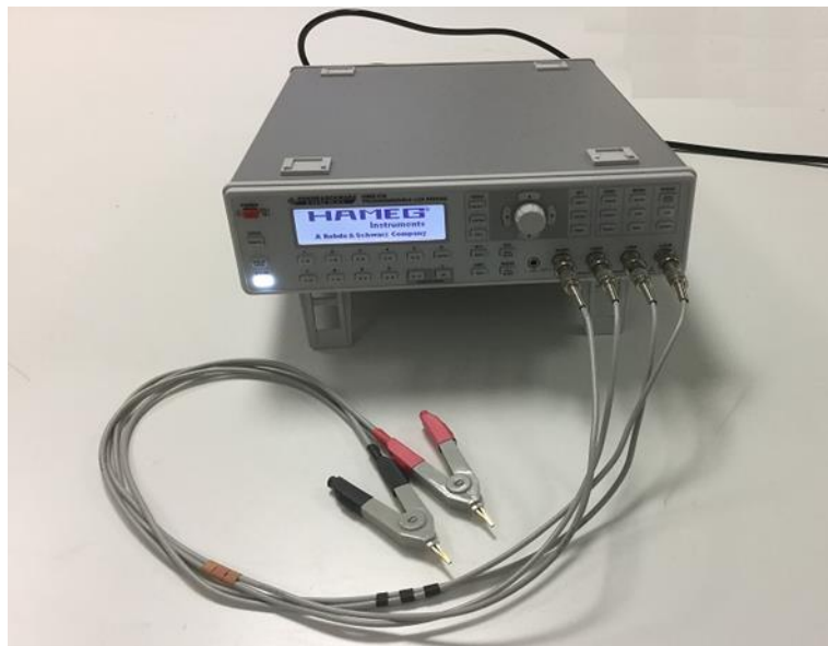
Figure 3.8 - LCR Bridge meter.
