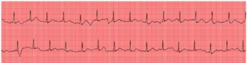
Figure 6.17 - ECG recorded from knitted SSB in the position of, (a) sitting, (b) walking, (c) arm moving position.
