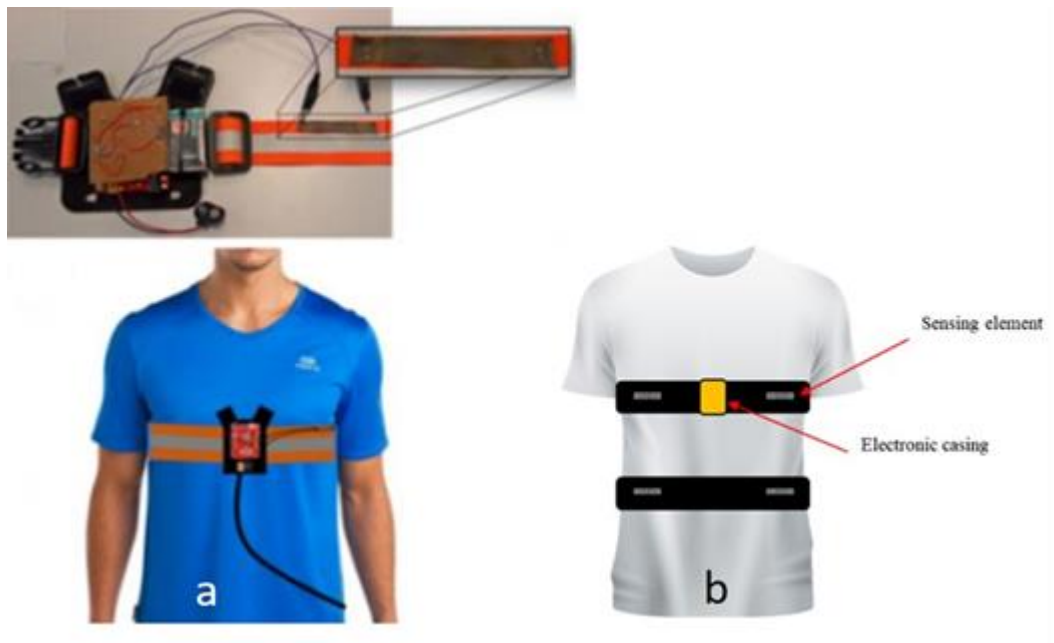
Figure 1.10 - Respiratory monitoring based on piezoresistive sensing, developed by a) Molinaro [23], b) Di Toccowe [24].
