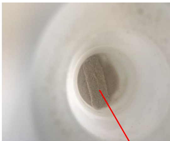
a) 4000 ppm, 100-315 \mu\text{m} Ayrshire limestone, pH4
