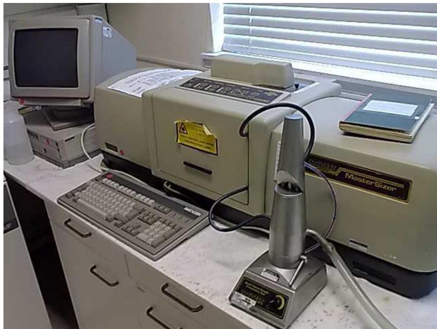
Figure 6.7. Particle Size Analyser - Malvern MS-20
