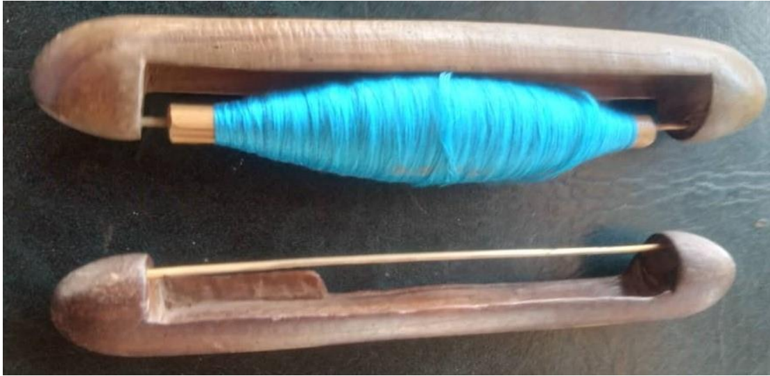
Figure 5:6: Two shuttles with one inserted with yarns-wrapped bobbins ready as the weft
